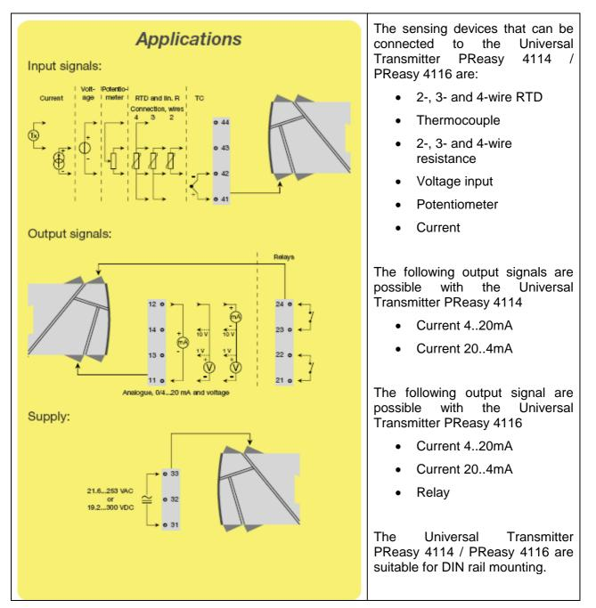
Figure 2: Input configurations with Universal Transmitter PReasy 4114 / PReasy 4116
