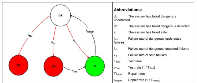
Figure 3: Markov model for a 1001D structure
